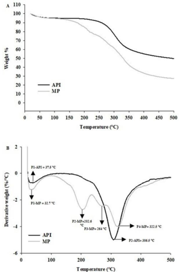
Figure 3. (A) Thermogravimetric analysis (TGA), and (B) derivative (DTG) of mantle protein (MP) and actomyosin-paramyosin isolation (API) from giant squid (*Dosidicus gigas*).
