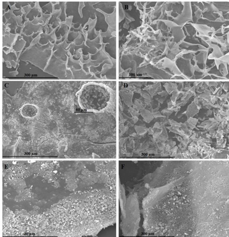
Figure 4. Scanning electron microscopy (SEM) micrographs of mantle protein (MP) and actomyosin-paramyosin isolation (API) from giant squid (*Dosidicus gigas*). (A) sol of API, (B) gel of API, (C) and (E) sols of MP, (D) and (F) gels of MP.
